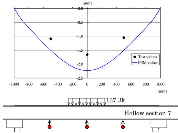
Fig. 11 Vertical deflection of the bottom flange of the aluminum deck [Hollow section 7]
