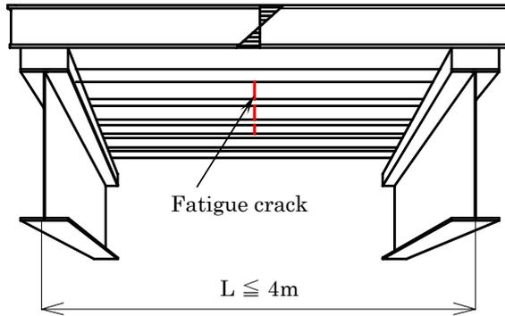
Fig. 5 Fatigue crack initiated on bottom flanges in the bridge-longitudinal direction
