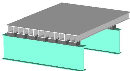
Fig. 2 Aluminum deck of open-hollow sections
