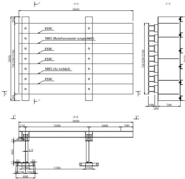
Fig. 8 Test specimen
