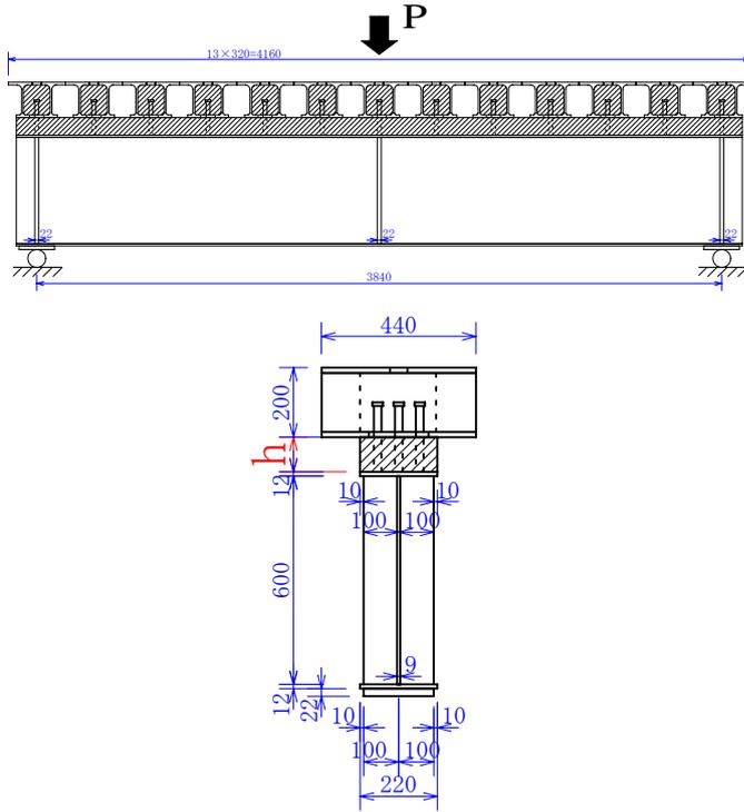
Fig. 17 Test specimen
