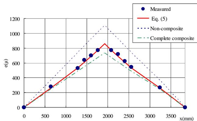
Fig. 20 Distributions of strain on the bottom flange of the steel girder [Specimen IV,  $P=495\text{kN}$ ]
