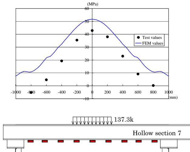
Fig. 13 Bridge-transverse stress on the bottom flange of the aluminum deck [Hollow section 7]
