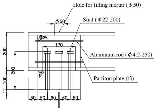
Fig. 7 Connection of the aluminum deck to the top flange of the steel girder
