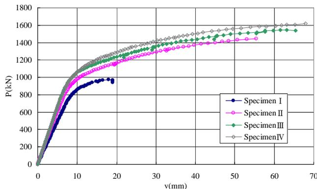
Fig. 19 Relation between load and deflection at the span center
