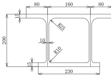
Fig. 6 Cross section of the extrusion
