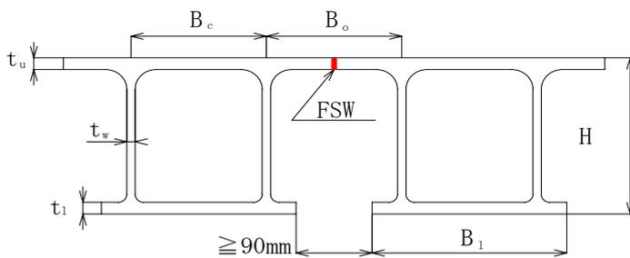
Fig. 3 FSW at the ends of the overhangs of extrusions
