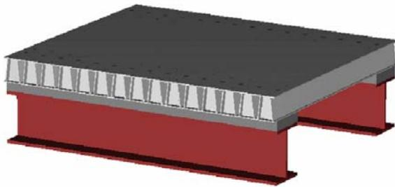
Fig. 1 Aluminum deck of hollow sections
