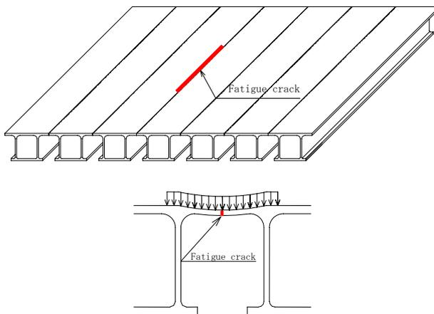
Fig. 4 Fatigue crack initiated along the FSW-joining line of a top plate
