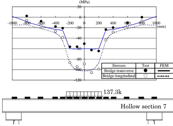
Fig. 14 Bridge-transverse and -longitudinal stresses of the top plate of the aluminum deck [Hollow section 7]
